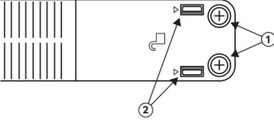
**EN** Remove terminal covers by unscrewing the clamp screws (1) and inserting a small flat-bladed screwdriver into the locking slots (2).
