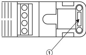
**EN** Wire in terminals using the wiring diagram on page 2 as a guide. The screw terminals are suitable for solid core or stranded cable up to 2.5mm<sup>2</sup>. Maximum cable OD 10mm.
