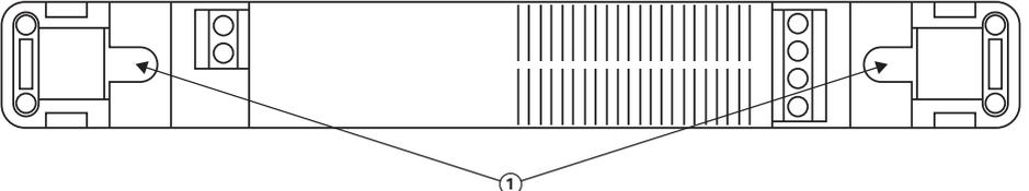
**EN** This standalone version is suitable to be mounted remotely. Mount the product in the chosen location, using the fixing slots (1) with M4 screws.
